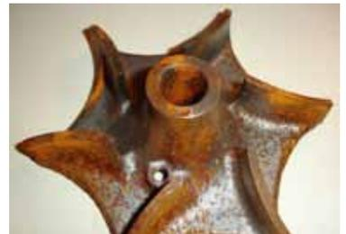
A severely rusted cast iron impeller.
