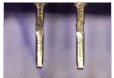
Cleaned sensor leads.
