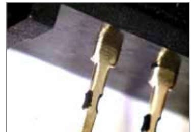
Black copper oxidation on contact leads.
