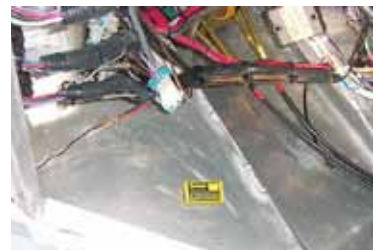
Zerust VC2-1 Vapor Capsules prevented corrosion and eliminating electrical problems in boat battery compartments.
