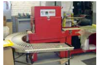
An L-Bar sealer used to package metal parts in Zerust VCI Film tripled hourly outputs.
