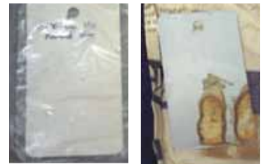
ASTM D1735 humidity chamber testing. Left; a steel panel protected by Zerust Film is corrosion free after 30 days. Right; a steel panel protected by competitor VCI paper has rust after 3 days.
