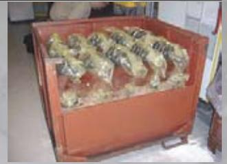
Gears packed in a ZERUST® Ferrous crate liner that covers the interior dividers in order to prevent contact with corrosion-causing wood.
