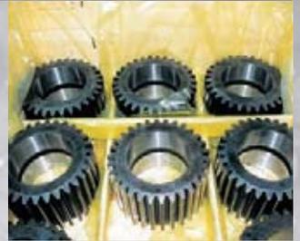
Small parts securely held by ZERUST® shrink film to ZERUST® treated cardboard.
