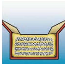
Insert additional ZERUST® packaging materials in the center of tightly packed parts to ensure protection throughout.
