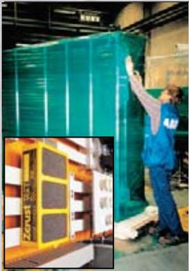
An electrical control cabinet protected inside by ZERUST® Vapor Capsules and protected outside with combination Zerust® Multimet/Anti-Static film.
