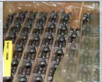
Stamped steel components being protected for sea freight with ZERUST® Multimet film.
