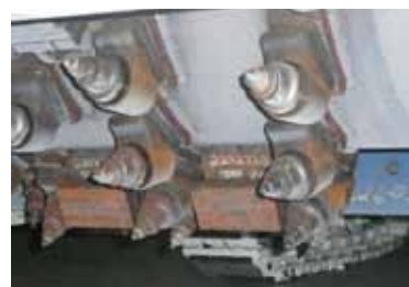
Non-critical area left unprotected by Axxanol Spray-G during shipment. Unprotected area quickly rusted.
