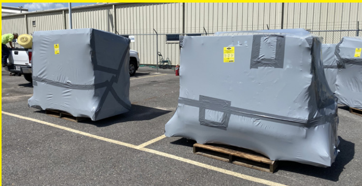
Large pieces of equipment shrink-wrapped in ZERUST® ICT®510-OPS Outdoor Preservation VCI Shrink Film for outdoor storage.
