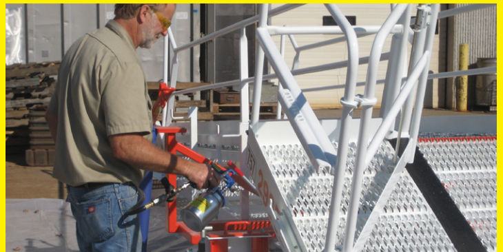
ZERUST® Axxanol™ Spray-G being applied to large equipment for outdoor storage, providing robust rust prevention.
