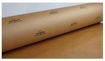
ZERUST® ICT®432-35P is a kraft packaging paper containing ZERUST® Vapor Corrosion Inhibitor Technology (VCI) coated with a 3/4 mil plain polyethylene coating on one side. The plain polyethylene coating provides the kraft paper with increased tear and moisture resistance. Place the plain kraft paper side facing the metal surface to allow the powerful vapor corrosion inhibitors (VCI) to protect ferrous and non-ferrous metal coils.
