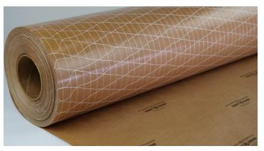
ZERUST® ICT®430-35SR Scrim Reinforced VCI Paper is a high-quality 35# kraft paper that is saturated on one side with proven ZERUST® corrosion inhibitors and laminated with a 3/4 mil polyethylene layer and fiberglass scrim on the backside to provide superior strength. Place the plain kraft paper side facing the metal surface to allow the powerful vapor corrosion inhibitors (VCI) to protect ferrous and non-ferrous metal coils.
