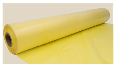
ZERUST® ICT®520-SRA VCI Plastic Scrim is a durable polyethylene fabric with woven strands for strength and tear resistance, as well as vapor corrosion inhibitor (VCI) corrosion protection. ZERUST® VCI Plastic Scrim is great for interleaving applications where strength and tear resistance are important. For example, use ZERUST® VCI Scrim to provide corrosion protection when stacking or wrapping metal coils during shipment and storage.
