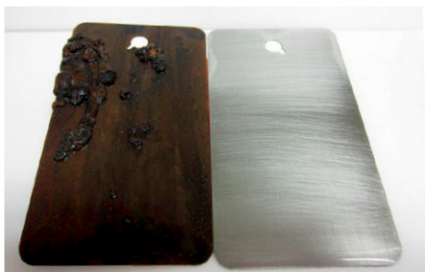
On the left: submerged in untreated water (60 ppm Cl - , 300 ppm CaCO 3 ), on the right: submerged in AxxaVis™ HST-10 treated water.
