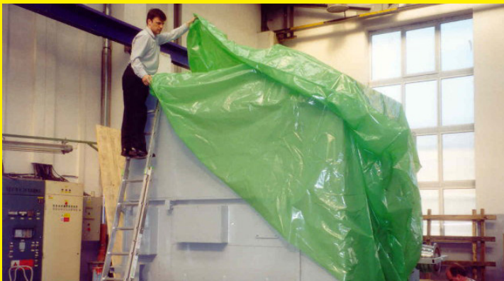
ZERUST® ICT®510-C Multimetal VCI Film protects an oversized piece of electronic equipment.
