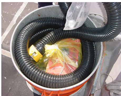
A bail-out pump motor protected by a ZERUST® ICT®510-C Ferrous Bag. Pump is corrosion-free and ready to use.
