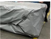
Lift the whole die and position the bottom sheet under the die set, then tack ZERUST® ICT®510-OPS sheeting with ZERUST® OPS Preservation Tape onto a painted die surface, up the side of the die. Use a neat tuck on the corners to lay as tight and flat as possible. Use the OPS Preservation Tape to hold it in place. Lower die and remove hoist attachments.
