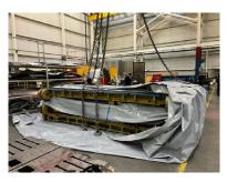
Place the top sheet of ZERUST® ICT®510-OPS over the top of the die, tape all overlapping sheets together, fold in the corners, and then tape with ZERUST® OPS Preservation Tape. Slowly heat shrink the film working from the edges, corners, and before careful application across the side and top panel. (Avoid burning through)
