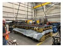
Lower the top die onto the bottom die, sandwiching the ICT®510-OPS sheeting between the dies. Next, place 2 ZERUST® ActivPak®-35 VCI Packets on either side of the die, around halfway on top of the ICT®510-OPS sheeting.
