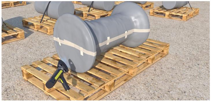
b. Use a shrink-wrap torch and/or gun to apply heat in steady strokes in a spray paint fashion. Be consistent and careful to keep the heat moving evenly on the surface.
